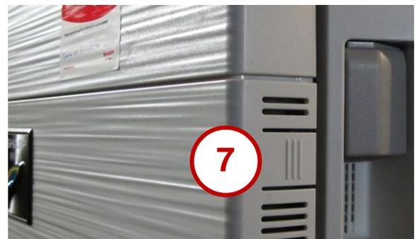
panel with the Sharp badge attached, it is part of the front surface of the copier. On each end of the panel there is a small area with vertical ribs (6) + (7). Using both hands at the same time (8) press these areas lightly towards the centre of the panel. The panel will then hinge downwards like the glove-box lid in a car.
