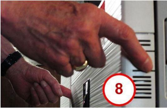
panel at the left-hand side of the area you have just revealed. It has the words MAIN POWER beneath it. The picture shows the switch in the OFF position. Press the top end of the switch to set it to ON.
